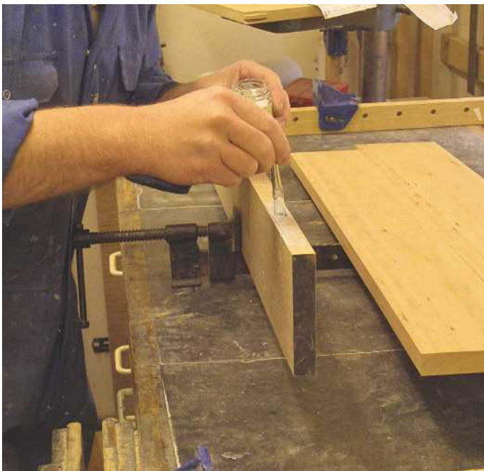
▲ Pic.2 Edge-joint the boards for the top with a rubbed joint. Apply glue to one edge which then needs rubbing against the mating part
